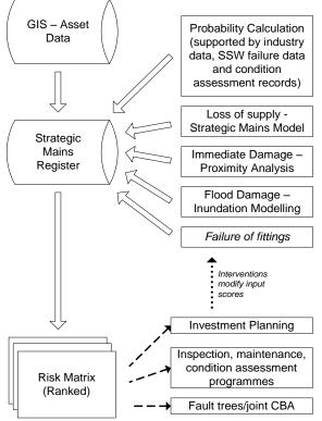
Figure 2: process diagram for trunk main register
