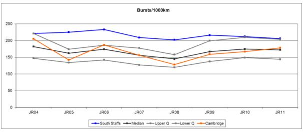
Figure 18: burst mains per 1000km of network (against industry reference)
