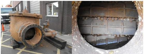
Figure 8: 36" multi-gate non-return valve removed during 2011
