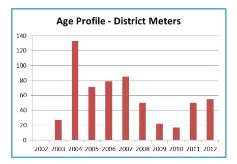
Mechanical meters do wear out over time. In AMP4 and AMP5, independent meter testing has been carried out by WRc NSF and TUV NEL to assess the performance of District Meters removed from service. The Company has tested 48 district meters in AMP4 and AMP5 to date to support the identification of an optimum District Meter replacement strategy.
