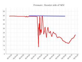
Figure 7: example 37m pressure surge near non-return valve
