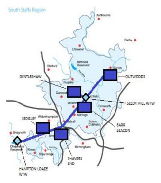
This diagram shows a simplified view of the trunk main spine running from south west to north east and the location of the two surface water treatment works at Hampton Loade and Seedy Mill.
