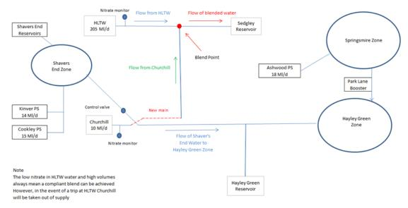
Figure 4, Schematic representing the construction of a new mains for blending.
