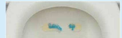
**Strip breaks in two:** It is likely you have a significant leak. Call an approved plumber to get it fixed.
