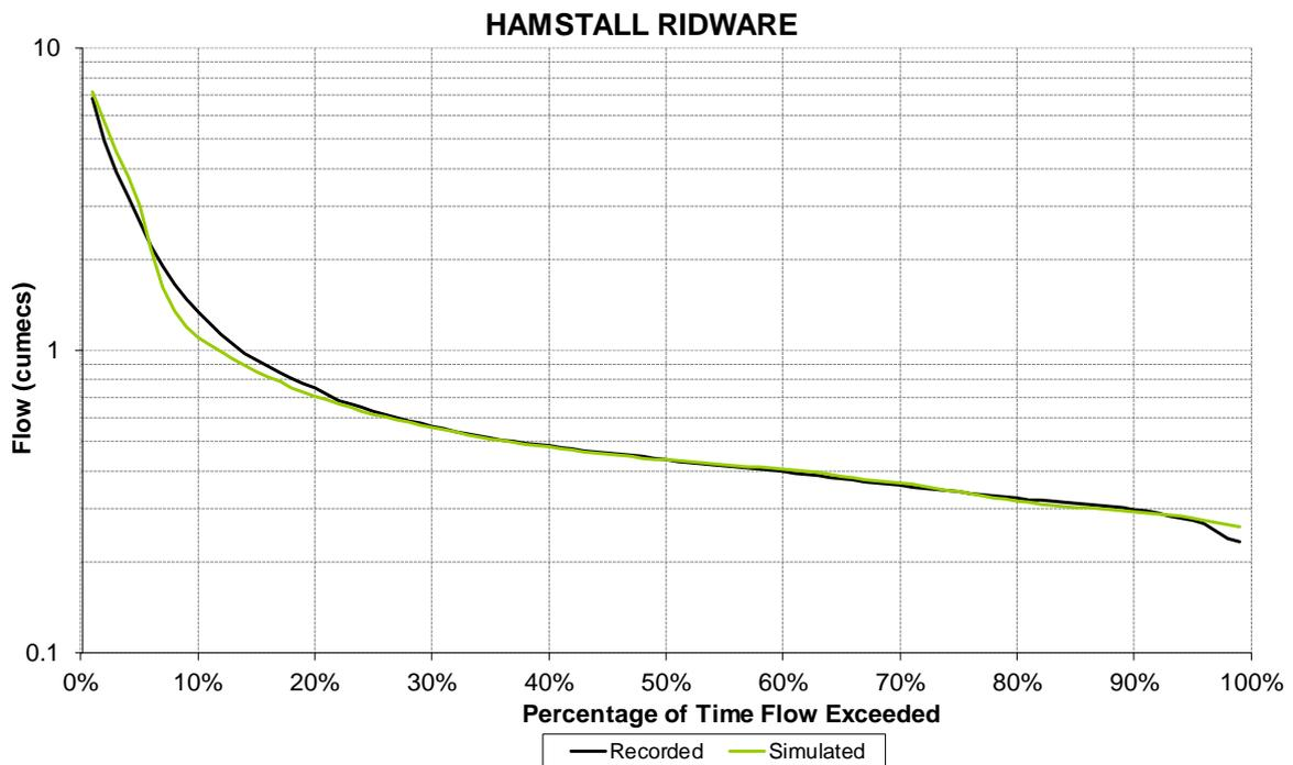
As can be seen there is a good match between the simulated and recorded FDCs at Hamstall Ridware for low and medium flows. Given that the flows from the downstream catchment will be used in Aquator to establish if there is enough water on the Blithe for pumping back into
