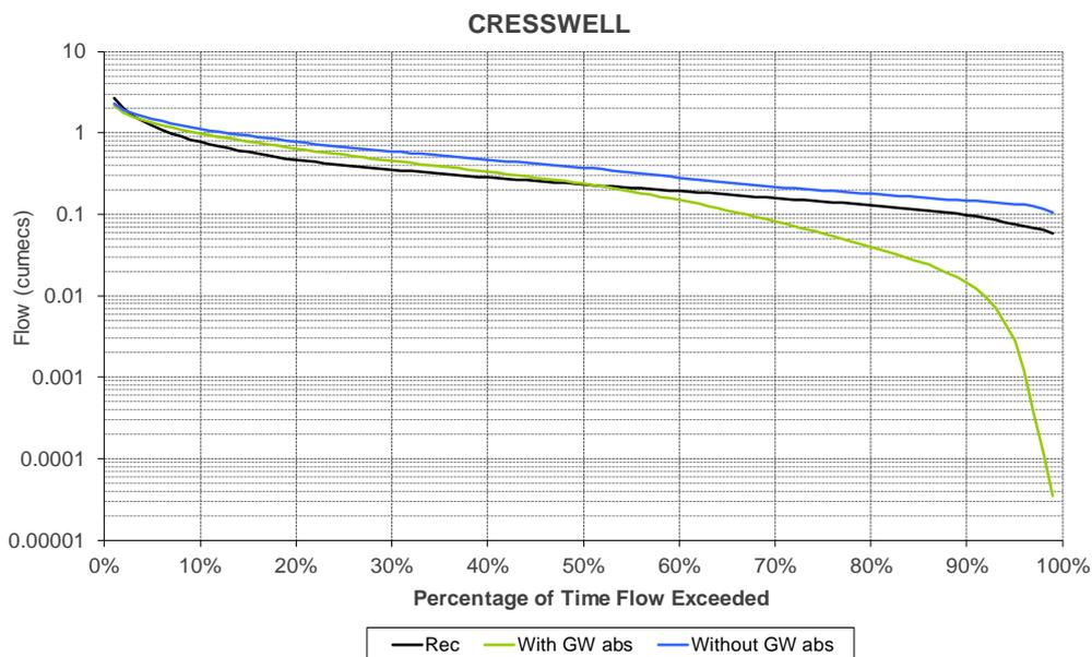
Mean annual flows at Cresswell were well estimated, which gives confidence in the simulated Blithfield flow series as it is going to be used in Aquator to feed a reservoir.
