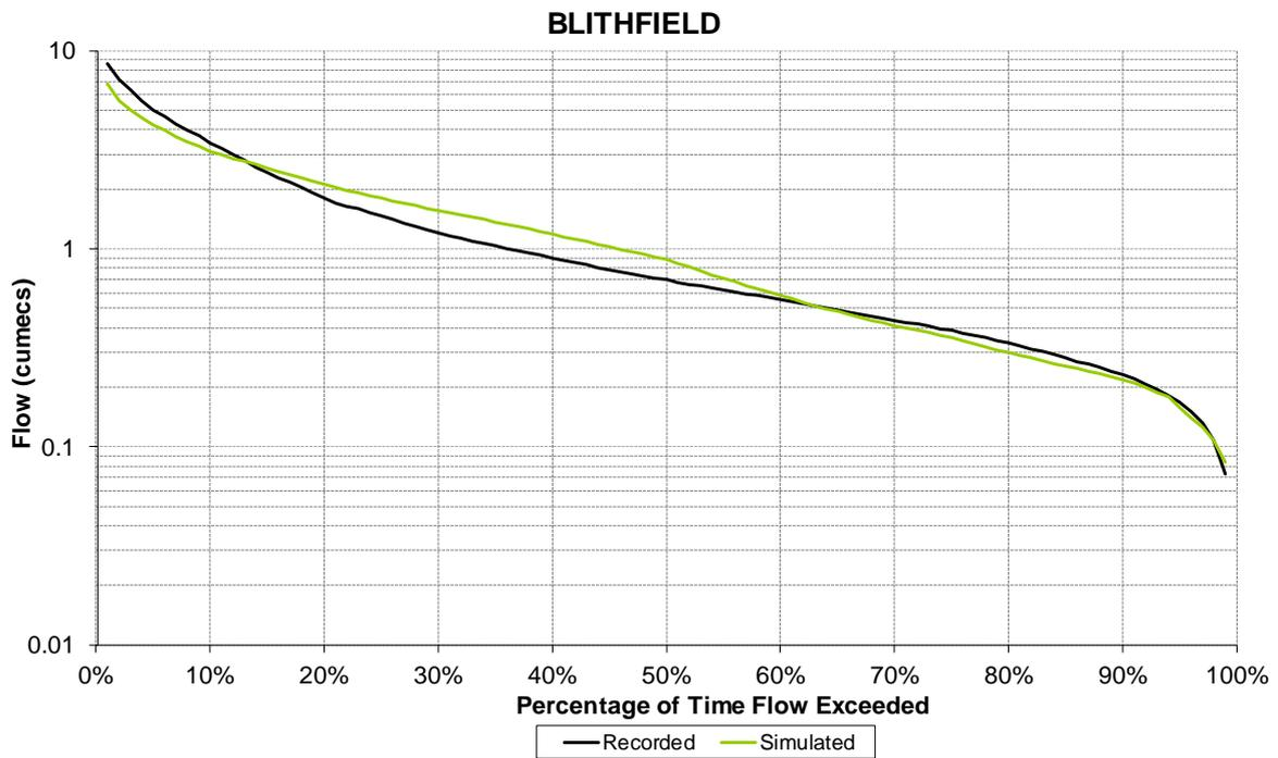
Figure 7: Comparison of FDCs in the downstream catchment (2005-2014)
