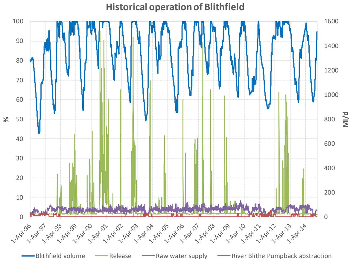
A preliminary derived inflow series was calculated but it was of poor quality, with numerous negatives and sharp oscillations due to the low accuracy of the water level meter, and possibly to some inconsistencies in other data. However, the estimated annual runoff is 353mm, which is consistent with the Cresswell value.
