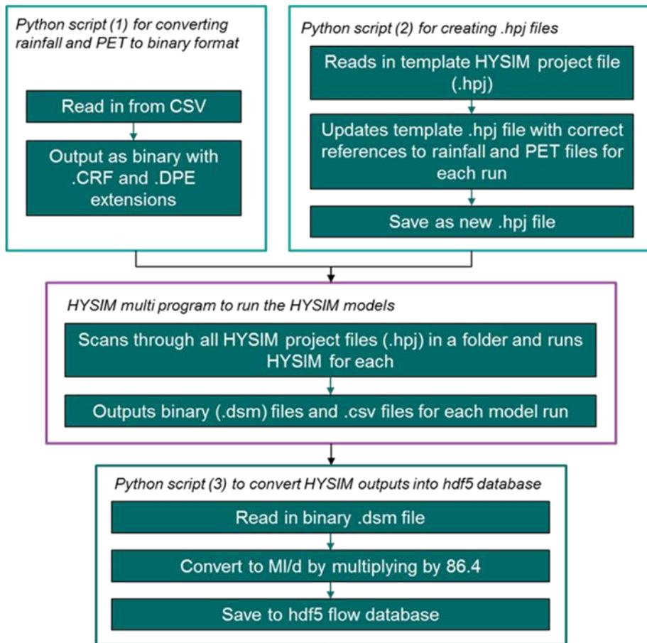
Figure 15: Flow chart for the HYSIM multi processing of synthetic droughts for a single catchment.
